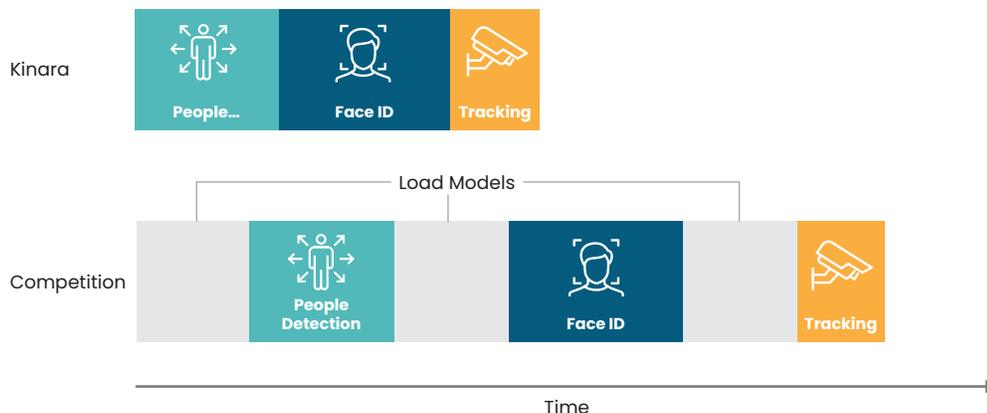
**Figure 2.** Kinara Ara-1 executes multiple models with no switching time overhead.
