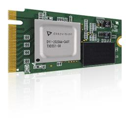
Kinara Ara-1 M.2 modules deliver plug-and-play compatibility to PCIe-enabled host systems. Start running inferences in minutes with a fully integrated module that includes the Kinara Ara-1 Edge AI processor, local memory and support circuitry.
